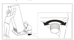
Slight unevenness in the floor can be leveled out using the front feet.
